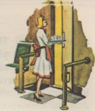
When someone nears the door, the light beam is interrupted and the door swings open.
